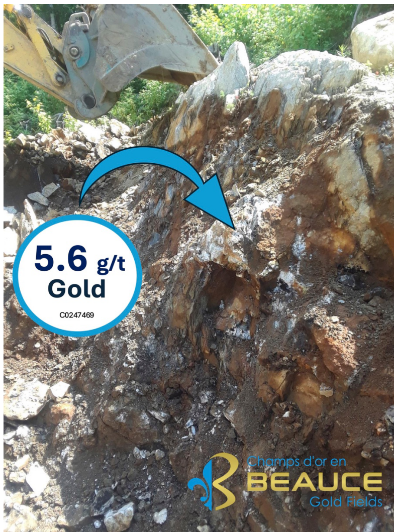
Image: stockwork vein of the Grondin outcrop, grade of sample C0247469
